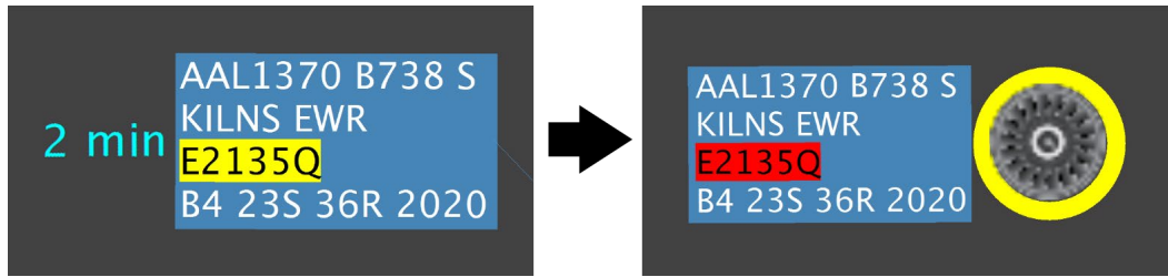
Figure 8.10. When a flight that is subject to both an EDCT (in this example, the EDCT is 2135 UTC) and an APREQ pushes back before the APREQ is scheduled, the field turns red and the EDCT continues to be displayed.
