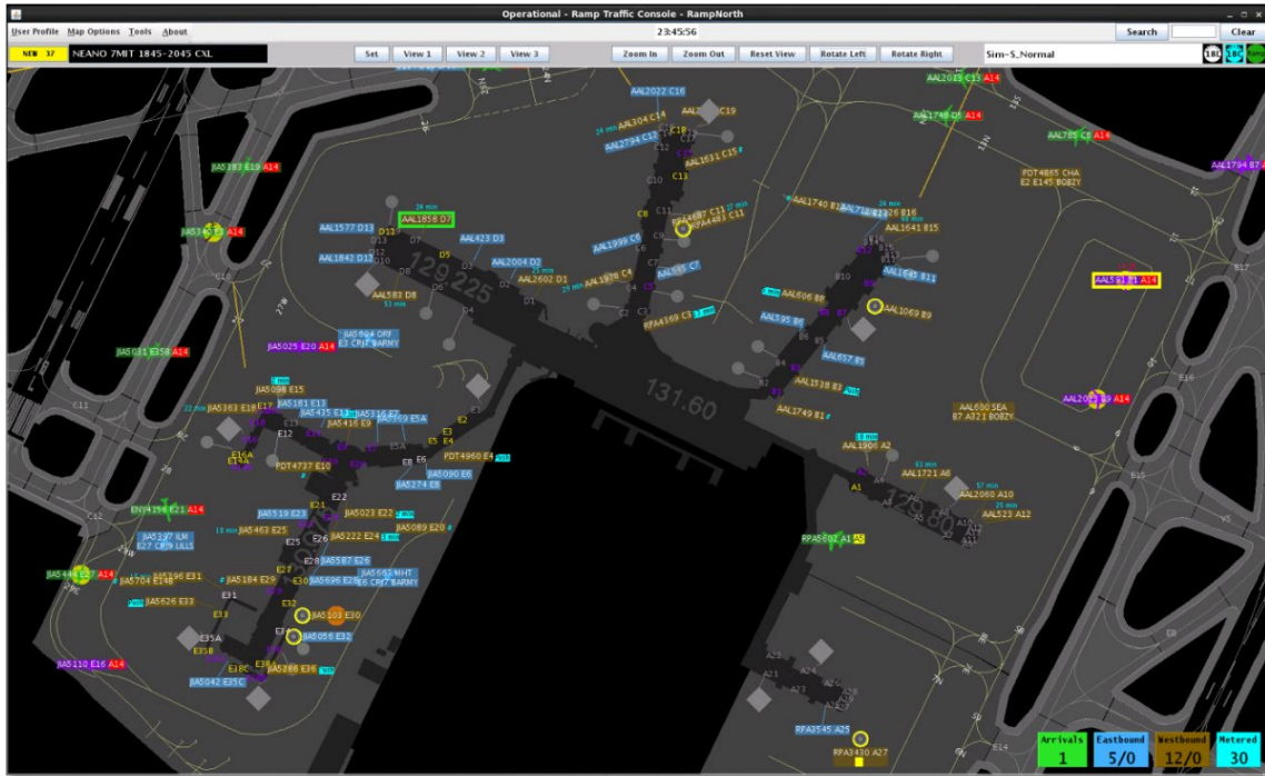
Figure 5.1. RTC map with flight strips and icons representing departure and arrival flights.
