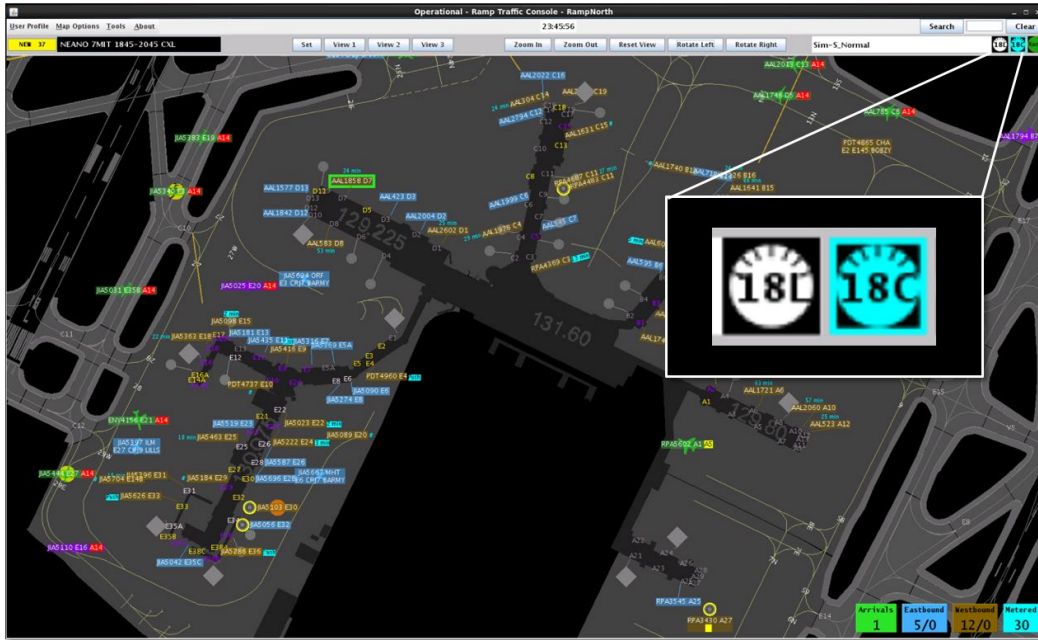
Figure 3.48. Runway SMP status icons. In this example, metering is active on Runway 18C.
