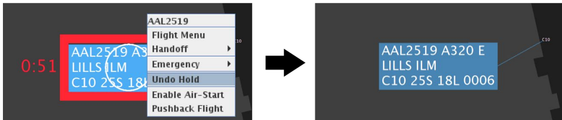
Figure 5.19. Right-click menu with “Undo Hold” selected (left). Red border and accompanying timer are removed from the flight strip (right).
