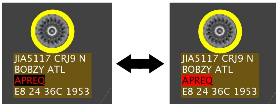
Figure 8.8. On the RTC display of the ramp sector owner, the APREQ field also flashes (inverted colors) until acknowledged.
