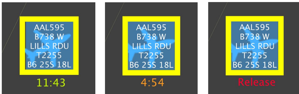
Figure 9.5. A hardstand release advisory is displayed for metered flights. The TMAT is displayed on the data tag (in this example, 2255 UTC).
