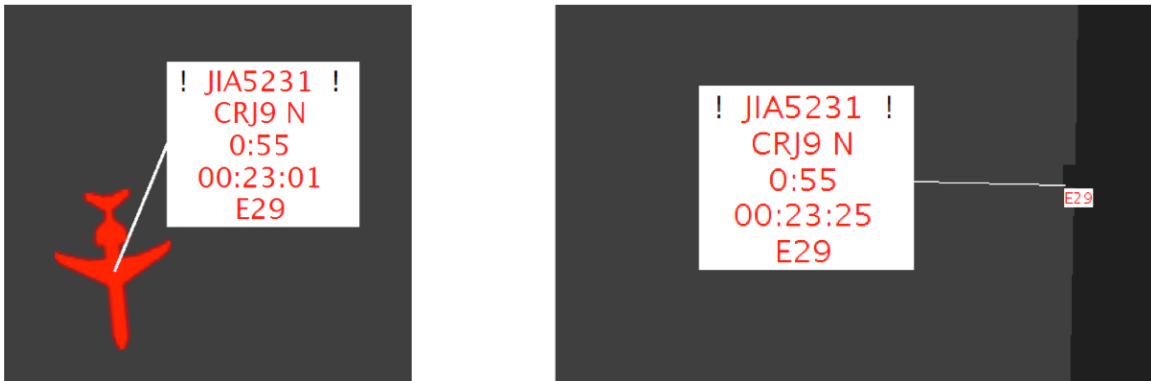
Figure 5.16. General emergency examples: Flight icon with attached data tag (left). Flight strip tethered to gate (right).
