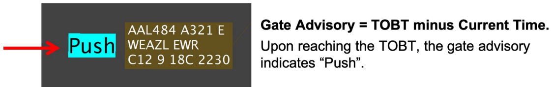
Figure 4.12. When the remaining Scheduler-recommended gate hold runs out at the TOBT, dashes (“--”) are displayed in the Hold column. At TOBT, gate advisory next to the flight strip displays “Push.”
