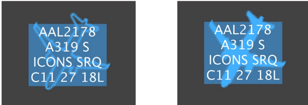
Figure 5.32. Departure flight: Not tracked by surveillance displayed as a hollow flight icon (left) and tracked by surveillance displayed as a solid flight icon (right).
