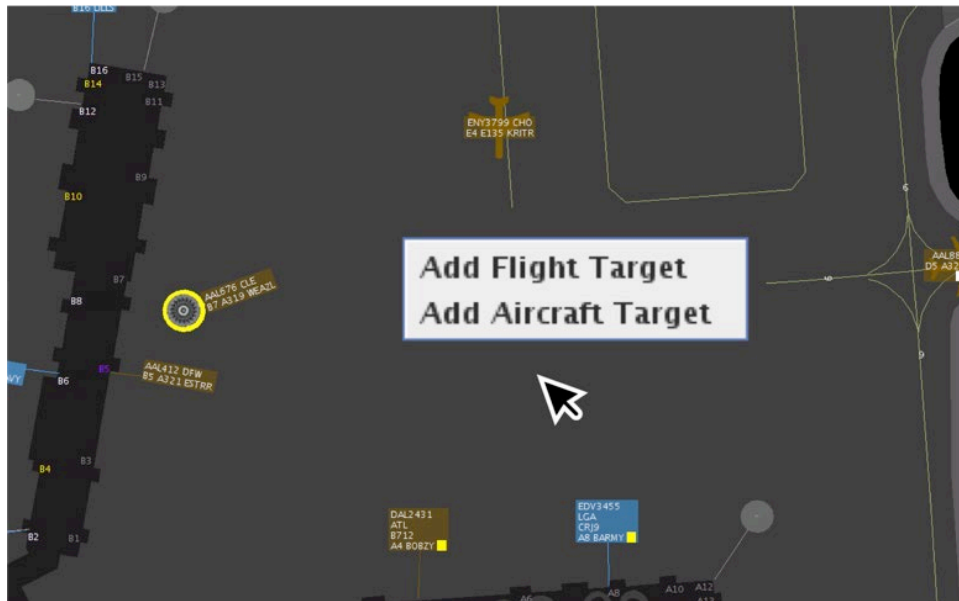
Figure 6.1. Right-click on an empty area of the map to show the target creation menu.
