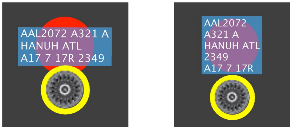
Figure 5.61. Examples of Long On Board (LOB) indicators displayed in the pushback/spool-up state (e.g., red indicators = 120+ minutes).
