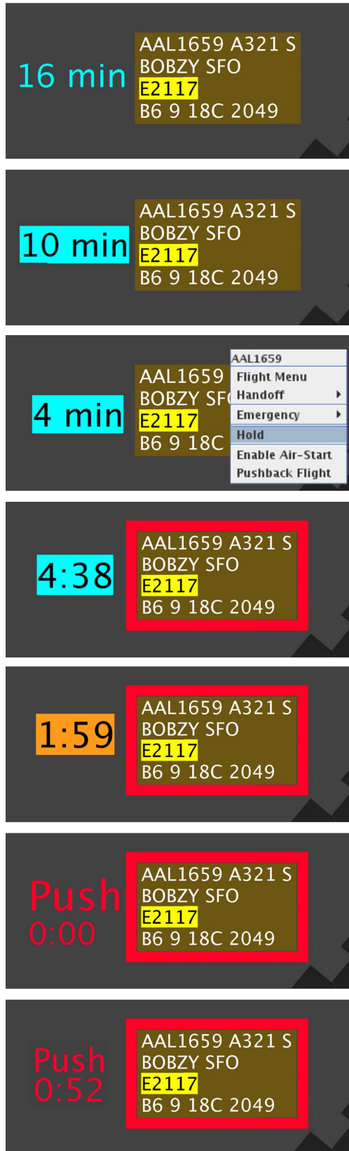
Figure 8.17. EDCT and APREQ flights: Put on hold when flight deck calls “ready.”
