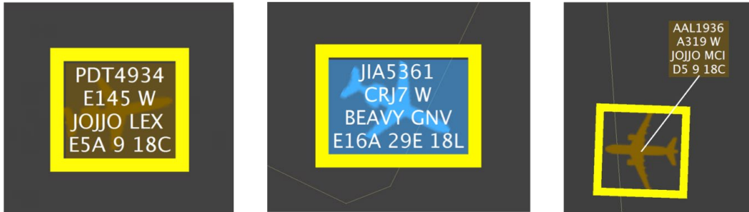
Figure 5.55. Departure flights holding in a hardstand are shown with a yellow border.
